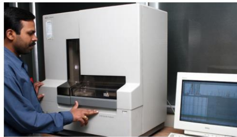
Genetic analyzer and 16 Capillary DNA sequencer and profiling equipment at the Centre for DNA Fingerprinting and Diagnostics lab in Hyderabad. FILE PHOTO
