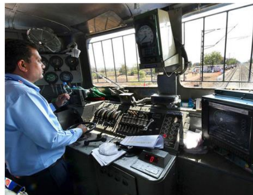
Safe and sound: The protection system alerts the pilot to red signals and applies automatic brakes if necessary. THE HINDU
