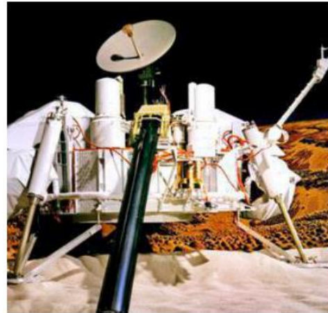
A model of NASA's Viking 1 lander, which became the first spacecraft to land on Mars in 1976. It was designed and operated to facilitate planetary protection. FILE PHOTO
