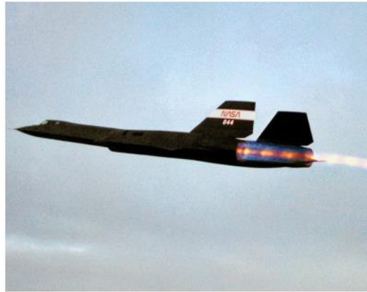
An SR-71 Blackbird takes off from the Dryden Flight Research Centre, California, on March 9, 1993. Shock diamonds are visible in its exhaust. NASA
