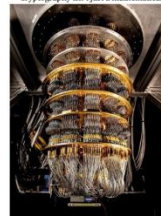
A cryostat refrigerator for cooling quantum computing chips at Google's Quantum AI lab in Santa Barbara, California, U.S. 10/17/2023
