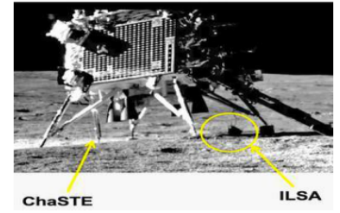
This image shows the ChaSTE instrument. ISRO
