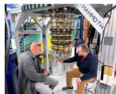
Google Quantum AI's Hartmut Neven (L) and Anthony Megrant (R) examine a cryostat refrigerator for cooling quantum computing chips at Google's Quantum lab in Santa Barbara, California. REUTERS
